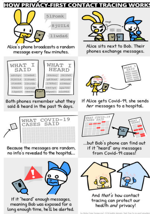
Figure 1: Decentralized contact notification server architecture
