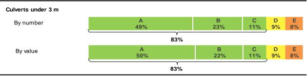
Across the road network, most (83% according to both length and value) culverts less than 3 m wide are in good condition and require no major short-term interventions. Culverts in poor and very poor condition (GCI of D or E) need to be monitored very closely, since they will require repair, rehabilitation or reconstruction in the coming years.
